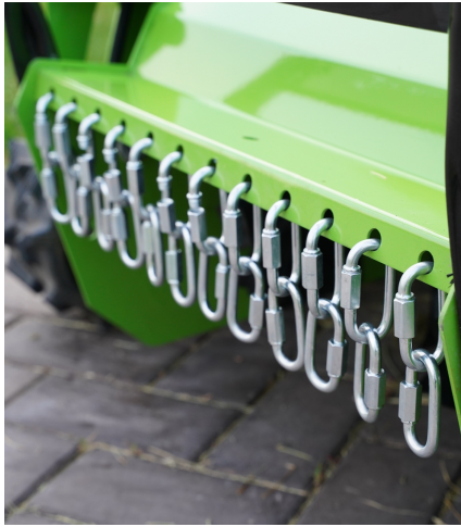
The front anti flying metal curtain prevents stones and blades from splashing, making mowing safer.
