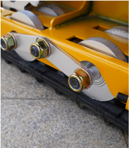
Double layered support wheel design ensures more stable machine operation.
