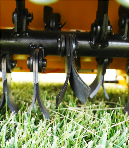
Using 16 sets of high-strength manganese steel blades, it is durable and long-lasting.
