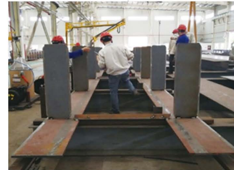
Install transverse stiffeners
